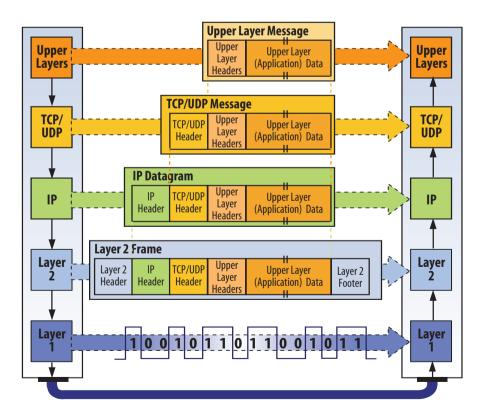
Figure 3: Overhead and Data at Each Layer
